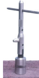
5. Attach tool. Turn clockwise to remove anchor.
