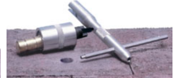
6. Place square tip of stud into tool to remove old anchor from extractor.
