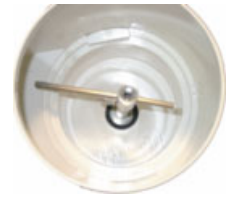
Hold plugs in place for vacuuming
