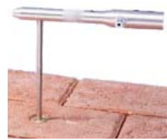
Raise/lower safety cover anchors (1/4" and 3/16" hex)
